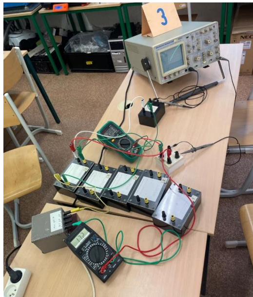
Figure 2. Experimental setup used for measuring the primary magnetization curve
